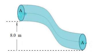
17. At the lower end of the pipe below the water speed is 6 m/s. At the upper end the speed is 9 m/s. The upper end of the pipe is 2 meters higher than the lower end. How much higher is the pressure at the lower end of the pipe?
