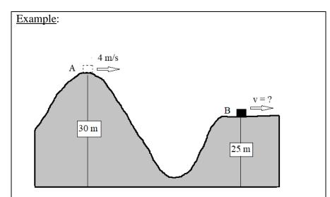
A cart at Point A, 30 meters above the ground, is initially moving at 4.0 m/s on a frictionless roller-coaster. What will be its speed when it reaches point B, 25 m above the ground?
