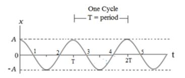
The largest positive velocities occur when the object is moving to the *right* through x = 0, such as at points 2 and 4. Maximum negative velocities occur at points 1, 3, and 5, when the object is moving to the *left*.
