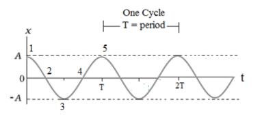
T = "Period" of the motion. It's the time it takes to complete one cycle of motion.
